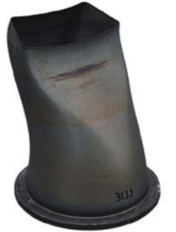
Mock-up sample of the outer shell of gas collector GTE-65.1 Stainless steel. Weight – 12 kg. Manufacturing time – 15 hours.
