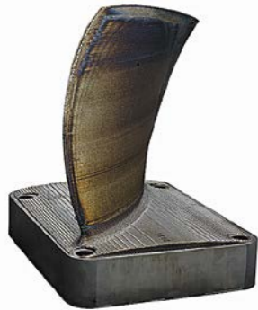
Blade. Stainless steel. Weight – 45 kg. Manufacturing time – 60 hours.
