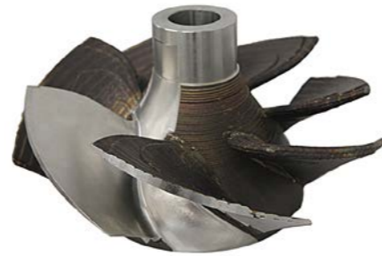
Billet of impeller water-jet propeller Stainless steel. Weight – 27 kg. Manufacturing time – 32 hours. Finishing machining is shown
