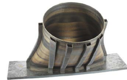
External housing of gas collector GTE-65.1 Stainless steel. Weight – 33 kg. Manufacturing time – 56 hours.
