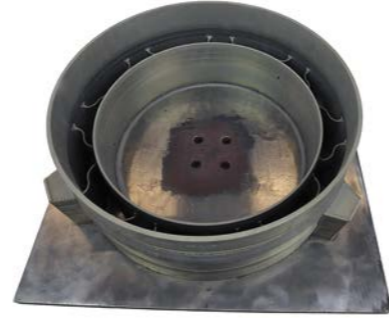
Gas collector inlet ring GTE-65.1 Heat-resistant nickel alloy. Weight – 15 kg. Manufacturing time – 37 hours.
