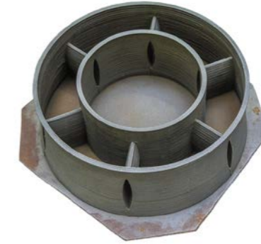
Mock-up of the center support. Heat-resistant nickel alloy. Weight – 23 kg. Manufacturing time – 29 hours.
