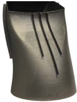
Mock-up sample of outer gas collector shell GTE-65.1 Stainless steel. Weight – 20 kg. Manufacturing time – 20 hours.
