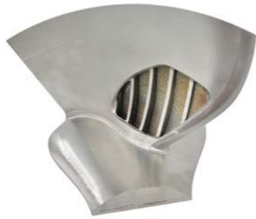
Topologically optimized blade of water-jet propeller Stainless steel. Weight – 12 kg. Manufacturing time – 12 hours.
