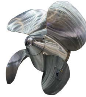
Propeller with topologically optimized hollow blades. Stainless steel. Weight – 160 kg. Manufacturing time – 100 hours.
