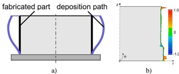
**Figure 10.** Scheme of fabrication part deviation from deposited part (a) and distribution of mismatch between required model and build part obtained using optimised deposition path (b)
