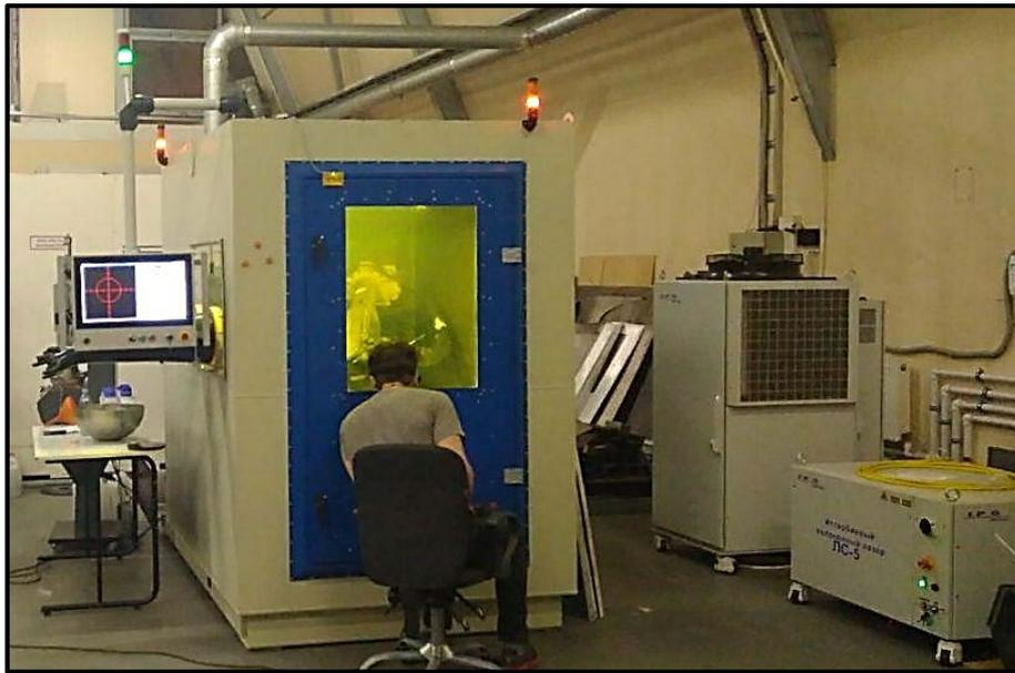
**Figure 1.** Laser metal deposition setup with an operator.
