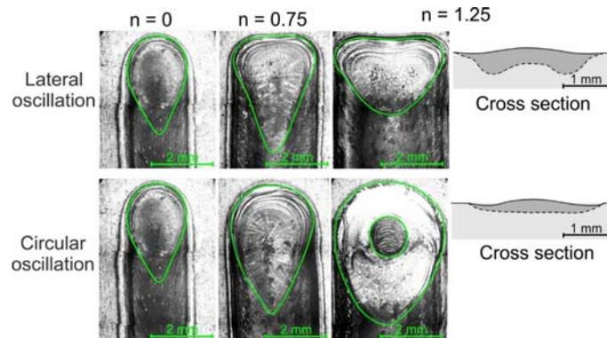
**Figure 7.** Effect of the oscillation amplitude on the molten pool shape.
