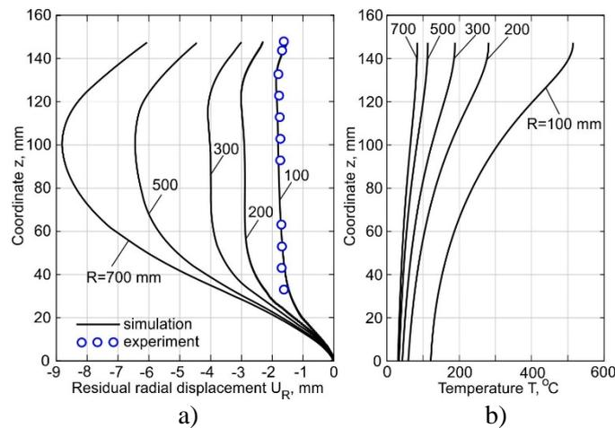
**Figure 7.** Residual radial displacement along the cylinder generator as a function of cylinder radius (a); Temperature distribution along the cylinder generator before the deposition of the last layer (b).
