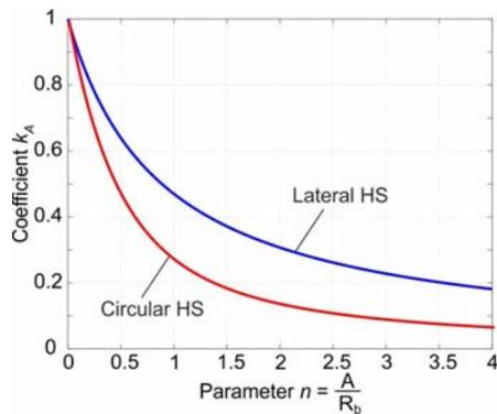
**Figure 6.** Coefficient  $k_A$  as a function of parameter  $n$ .
