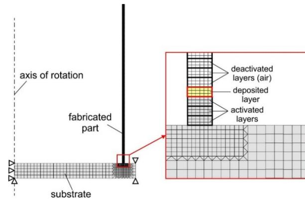
**Figure 5.** FE mesh and mechanical boundary conditions
