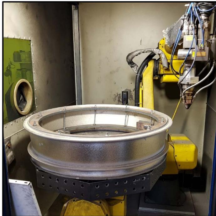
**Figure 4.** Photo of the deposited cylinder of Ti-6Al-4V with flanges
