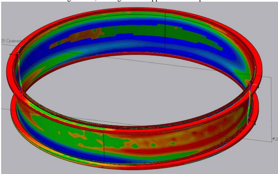
**Figure 11.** Distribution of mismatch between required model and build part obtained using optimised deposition path.
