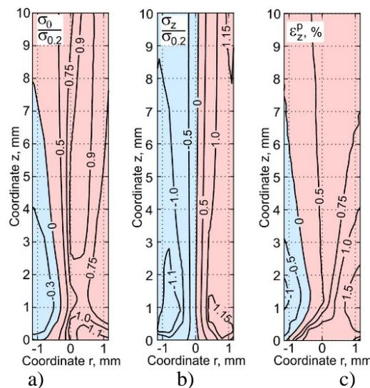
**Figure 8.** Distribution of normalised hoop stress (a), normalised axial stress (b) and axial plastic strain (c) in the sidewall cross section of the cylinder of 700 mm radius.
