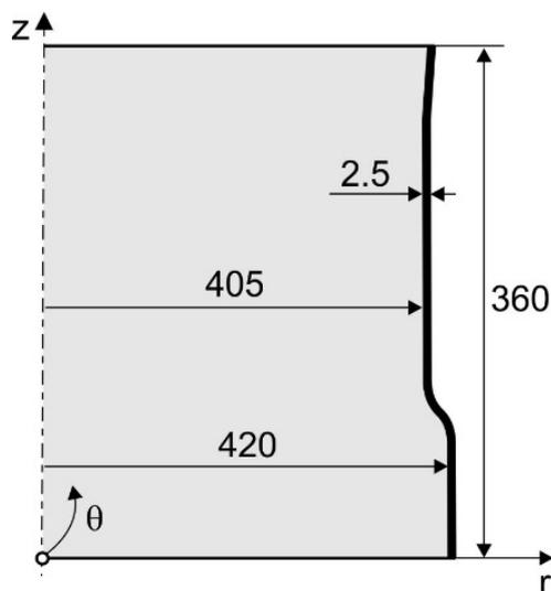
**Figure 3.** Scheme of the deposited cylinder of Ti-6Al-4V
