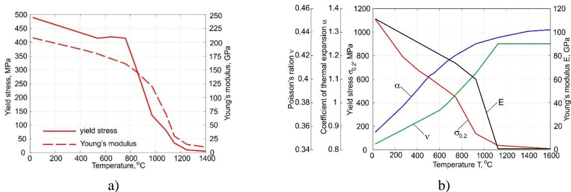
**Figure 6.** Temperature-dependent mechanical properties for IN625 (a) and Ti-6Al-4V (b).
