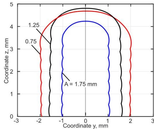
**Figure 10.** Effect of the amplitude of lateral oscillated laser beam on the cross section of the deposited wall.
