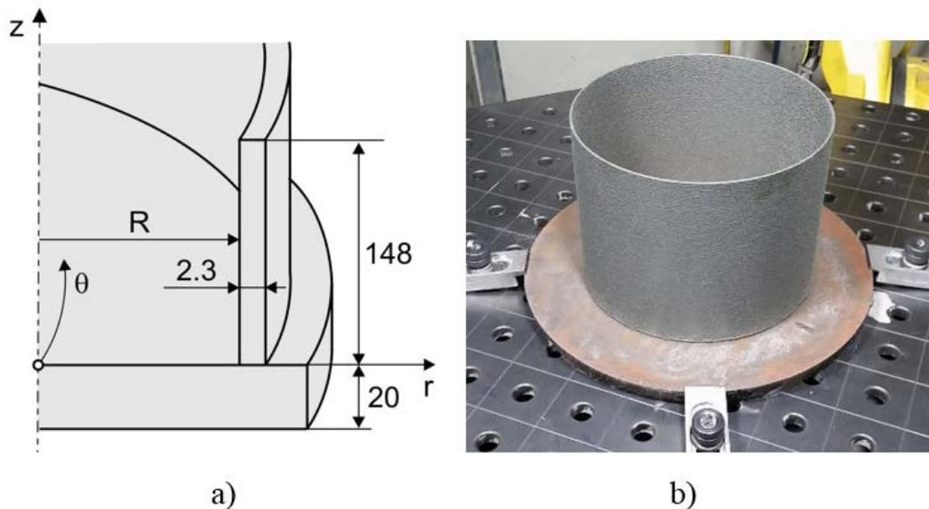
**Figure 2.** Schematic (a) and photo (b) of the deposited cylinder of IN625.
