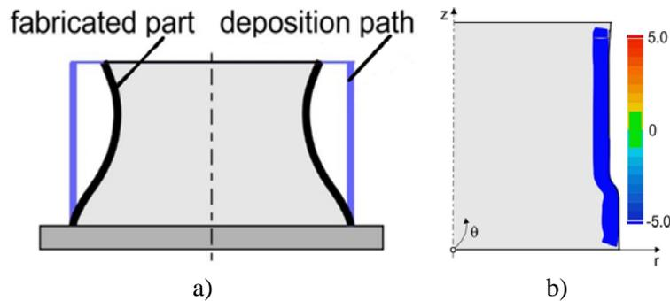
**Figure 9.** Scheme of fabrication part deviation from deposited part (a) and distribution of mismatch between required model and build part obtained using non-optimised deposition path (b)
